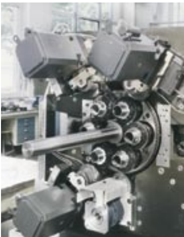
Auxiliary drive units for the speed-controlled direct drive in selected spindle positions.
