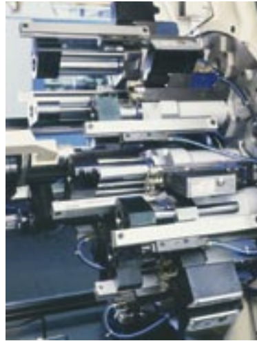
Drive housing with hydraulic endworking slide drives
