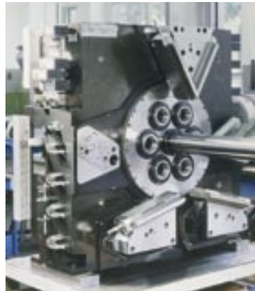
Spindle housing with drum and guide tube, cross slide support brackets and some of the slideways
