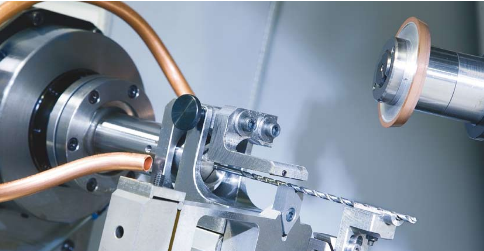
The patented work guide system WFS provides optimal guidance even for workpieces with a large L/D ratio (e.g. deep-hole drills)
