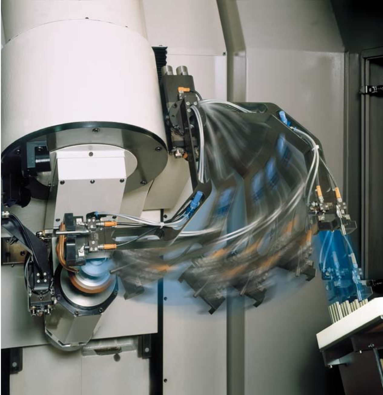
Automatic loading and un- loading of the workpieces by pick-Up loader
