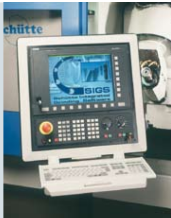
Siemens 840-D control system with SIGS user interface
