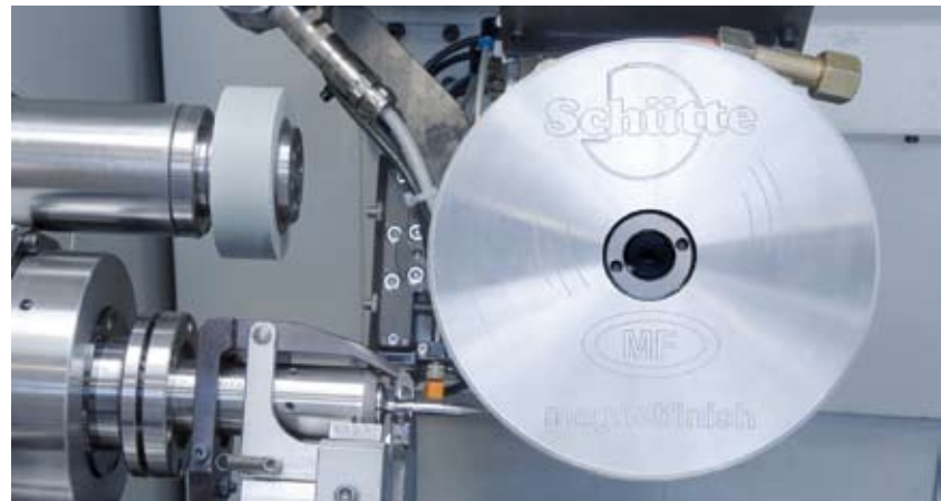
Cutting edge preparation on the machine, using the magnet-finishing process
